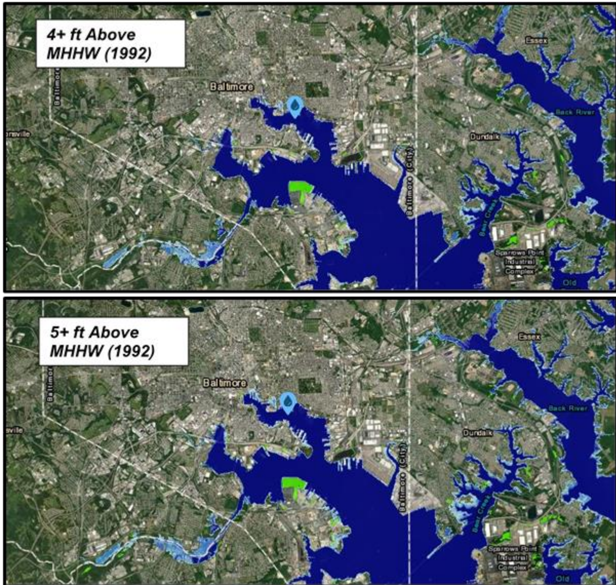
Figure 12. Sea Level Rise Viewer of Port of Baltimore Area. The top figure shows the Port Area at MHHW (1992) +4 feet of Sea Level Rise. The bottom figure shows the existing water level at Mean High Higher Water (1992) +5 feet (epoch: 1983-2001) (NOAA, 2020).
